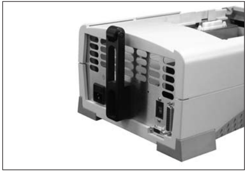
Fig. 2.3. Secure the support bracket to the rear of the iCycler chassis.
