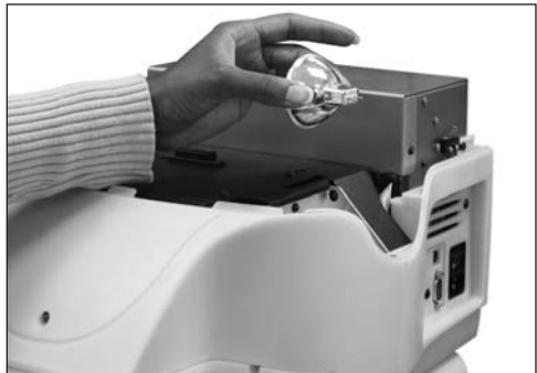
Fig. D.1. Replacing the lamp.
