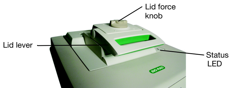
Figure 5. A top view of a reaction module.
