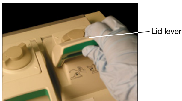
Figure 11. Push the lid lever down.
