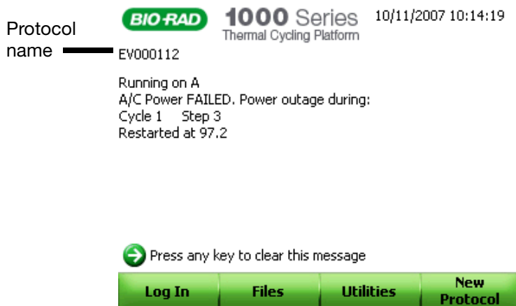
Figure 114. An error message alerting that the protocol was interrupted.
