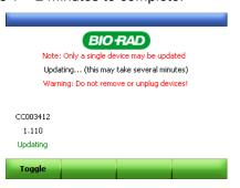
44) When the update has completed the system indicates "Update Complete! Please Reboot ALL Systems." Turn off the instrument, then turn it back on.
