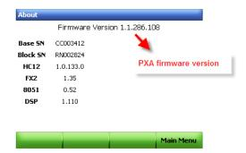
8) Record the firmware versions currently installed on your instrument in the table below:
