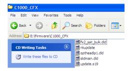
2) Copy the five firmware files onto an empty Bio-Rad USB Thumb drive (supplied with the instrument). Ensure there are no older versions of the firmware files on the thumb drive. When formatted correctly for firmware upgrade, the USB thumb drive will list the files exactly as shown in the figure below:
