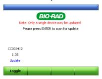
35) When ready, press **Enter**. The system scans the thumb drive for the necessary file (FX2\_SAT\_BULD.DLD). The message "Please press ENTER to begin update" is presented. Press **Enter**.
