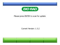
21) When ready, press **Enter**. The system scans the thumb drive for the necessary file (NKUPDATE.BIN). The system copies the update file to memory and then scans the file.
