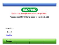
43) The update process will start. **Do Not** turn off power or remove any devices during this process. This process takes 1 − 2 minutes to complete.
