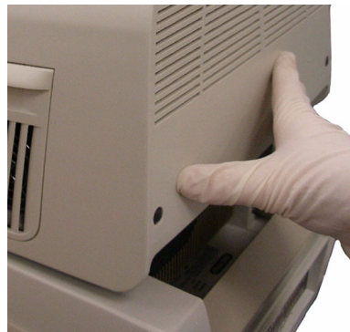
Figure 9. Push module forward until it stops moving or locks in place.
