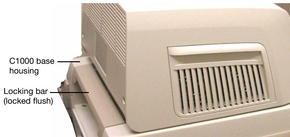
Figure 10. Locking bar in locked position and flush with housing.
