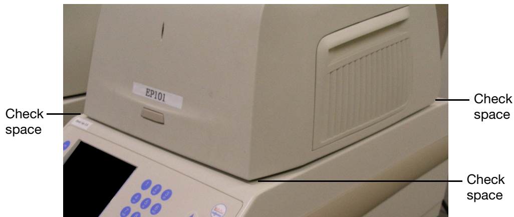
Figure 11. Check for even space between module and base, as shown here.
