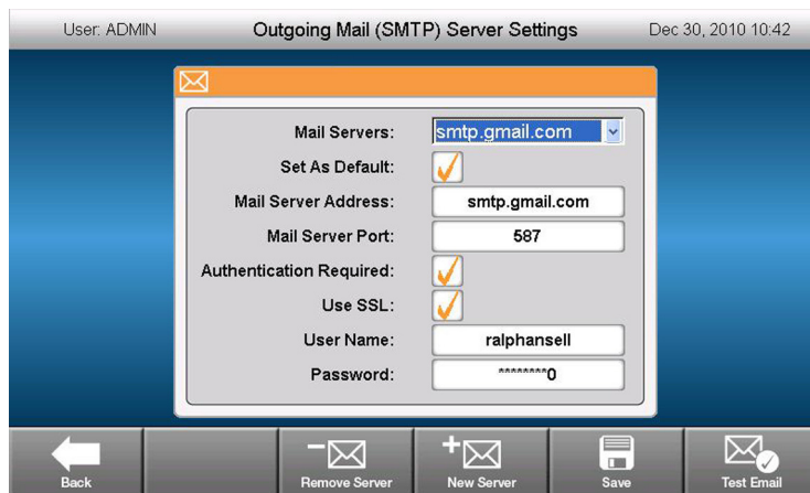
Figure 47. Gmail server is selected, user name and password have been entered, and this server has been selected as the default server for email communications.
