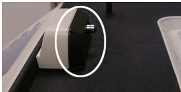
Figure 112. Optical module locking latch.
