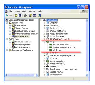
II. If you see the following screen, where there is only WinDriver listed under Jungo and MJ Real Time Detector USB Device and MJ Thermal Cycler are listed under the USB Serial Bus Controllers section, you must install the drivers manually. Please continue with step 18.
