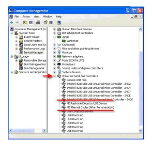
18) Right-click the MJ Real-time Detector USB Device driver under Universal Series Bus controllers and select Update Driver option.
