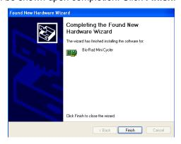
14) Repeat steps 10-13 for any additional new hardware installation screens that appear. Typically there will be two, one for the Bio-Rad Mini Cycler and another for the Bio-Rad Mini Optical Module.
