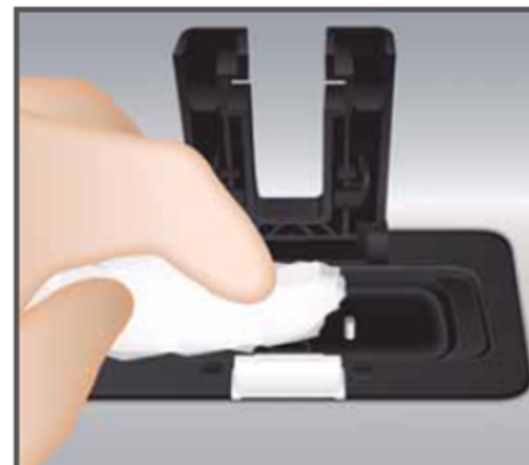
Figure 31 Dry the Wash Reservoir
