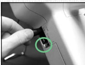
Allow the battery to charge for a full eight hours before using the instrument on battery power.
