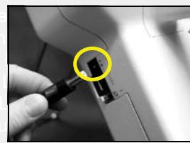
9 - Attach the AC power adapter connector to the instrument.
