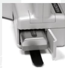
3 - Pull the battery release ribbon out of the cavity and place the battery on top of the ribbon.
