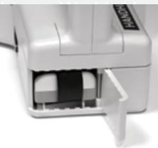
6 - Close the battery door so that it is flush with the bottom of the HANDHELD.
