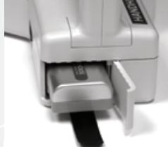
5 - Tuck the release ribbon over the top of the battery and into the cavity.
