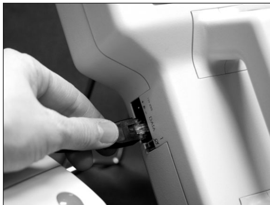
Figure 2-14 Attach printer cable to DATA port
