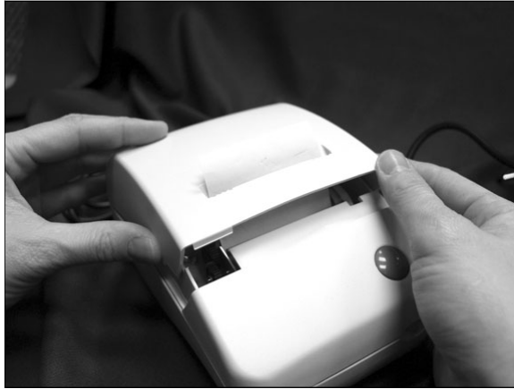
Figure 2-23 Feed paper through the printer's cover
