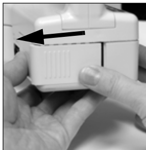
Figure 2-10 Unlatch Battery Compartment door
