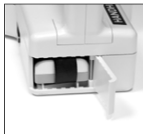
Figure 2-7 Tuck battery release ribbon
