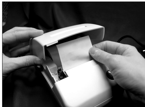
Figure 2-22 Preparing to feed paper through cover
