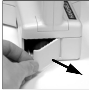
Figure 2-11 Open Battery Compartment door
