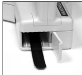
Figure 2-4 Pull Battery release ribbon out
