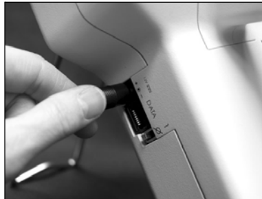
Figure 2-2 Inserting power jack.
