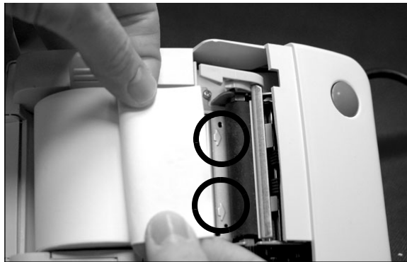
Figure 2-18 Printer paper guides (circled)
