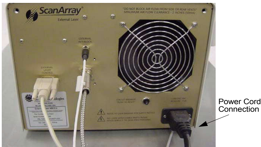
Figure 3-2 External Laser Rear Panel
