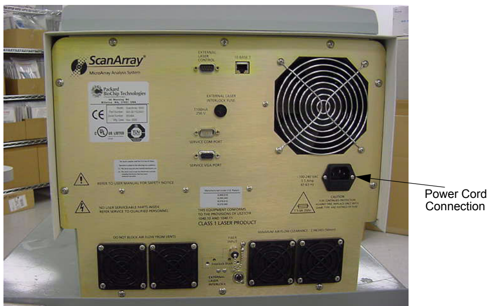
Figure 3-1 Rear Panel of the ScanArray Express Instrument
