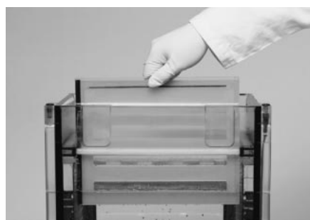
Fig 30. Inserting Precast Gel Cassettes into the Ettan DALT twelve Separation Unit.
