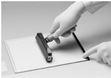
Fig 25. Pressing out air pockets between gel and glass plate.
