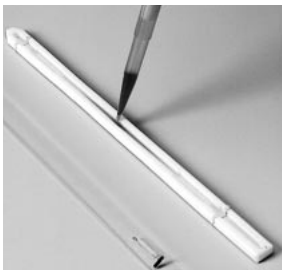
Fig 17. Applying rehydration solution into the strip holder.
