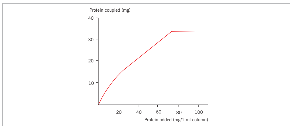
Fig. 60. Ligand coupling to HiTrap NHS-activated HP.
