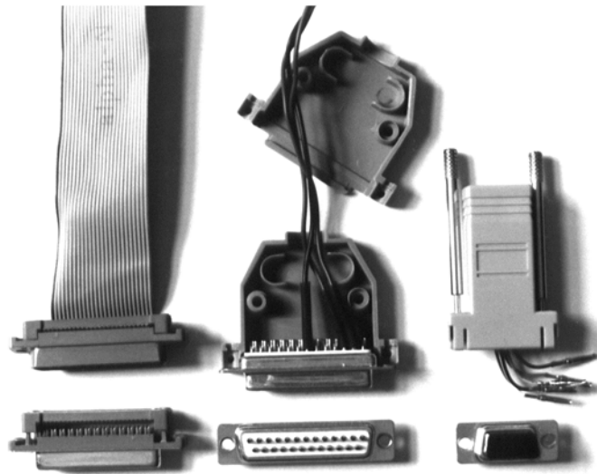
Figure 7-5: When making your own cables, there are several options for connecting the wires to the connector. From left to right: a ribbon cable clamps into an IDC (insulation displacement connector); individual wires solder onto solder-cup connectors; other connectors accept wires with crimp-on connectors.
