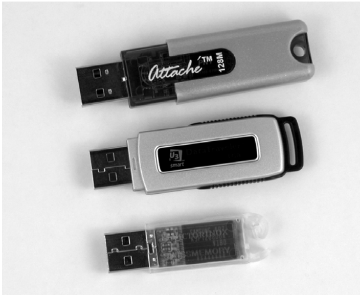
Figure 1-3: USB flash drives provide convenient storage that PCs and other USB hosts can access.
